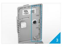
Inside the lid is a mounted PIR and two springs wired to the camera's sensors (PIR and touch). At the entry point of either side, a touch bar engages with the springs when the lid is closed.
