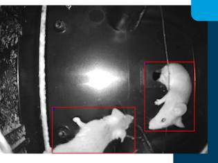
At the core of PestOptix is an artificial intelligence (AI) enabled cloud-based software. Similar to popular AI systems like Apple Siri® or Amazon Alexa®, PestOptix AI is comprised of sophisticated algorithms that have been trained to react to inputs. The AI software monitors the image inputs taken from camera sensors in traps in real time. When a pest enters a trap, PestOptix AI uses facial recognition algorithms to identify the pest type and alerts pest management professionals.
